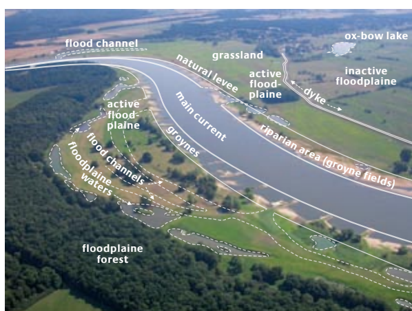
The system consisting of main current, river regulating structures and adjacent floodplain is the object under consideration (Photo: BFG)
